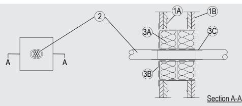
System tested with a pressure differential of 2.5 Pa between the exposed and the unexposed surfaces with the higher pressure on the exposed side.
