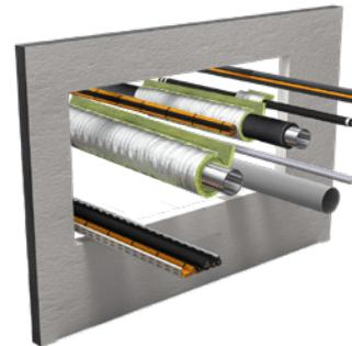
3. When additionally installing Nanosun<sup>2</sup>, HVAC split line combinations or HANSA-FLEX hydraulic hoses, apply the fire protection wrap DG-CR 1.5, when installing combustible pipes, apply the fire protection wrap DG-CR BS as necessary.
