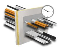
6. After the mortar residues have dried, remove them from cables, walls and floors, clean surfaces. Remove the protective sheets and ensure their proper disposal.
