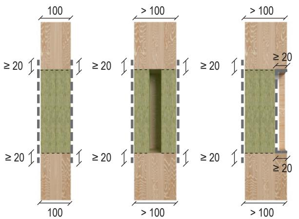
— = coated with FLAMMOTECT-A (dry film thickness ≥ 1.0 mm)
