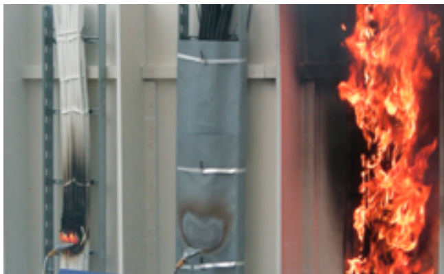
Comparative fire behaviour of cable trays (from left to right)
