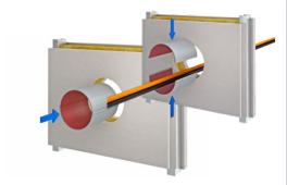
2. Seal the annular gap with NOVASIT BM / K2 or GFM.
