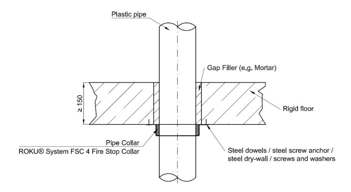
Penetration of pipes, floor installation - section view
