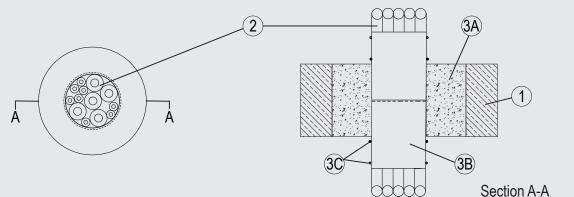
System tested with a pressure differential of 2.5 Pa between the exposed and the unexposed surfaces with the higher pressure on the exposed side.
